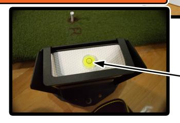
The level indicator is on the top of the device. You can make adjustments by adjusting the 3 legs of the device.
